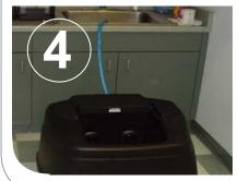
Route the discharge hose into a drain or sink.
